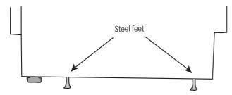
3. After the steel feet have been adjusted, screw down the two rubber feet tightly against the floor.
